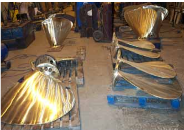
All blades are balanced before final inspection to ensure low levels of vibration in service
