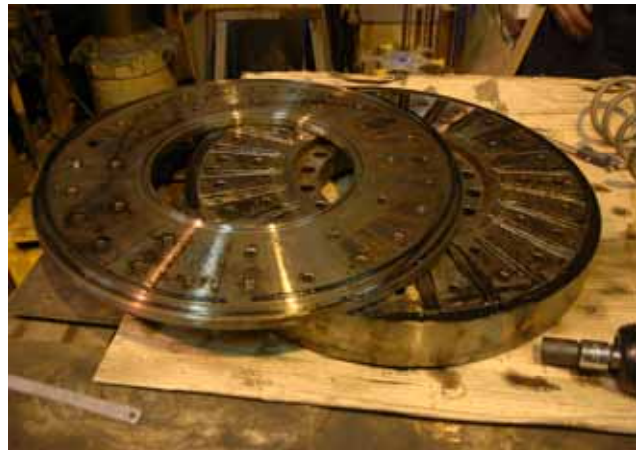
Damper awaiting stripping and cleaning during 30,000 hr inspection
