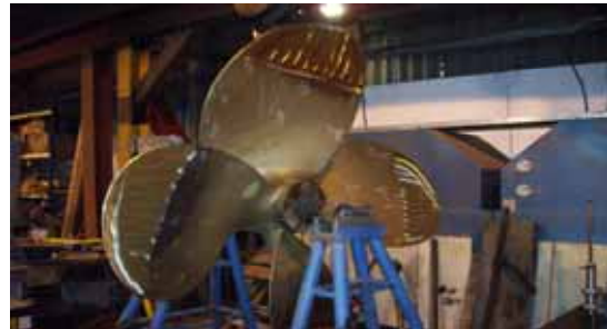
Surfaces are built up using TIG, MIG, and Gas welding techniques. selected to suit the specific propeller material. Post welding stress relieving and heat-treatment is carried out as necessary.
