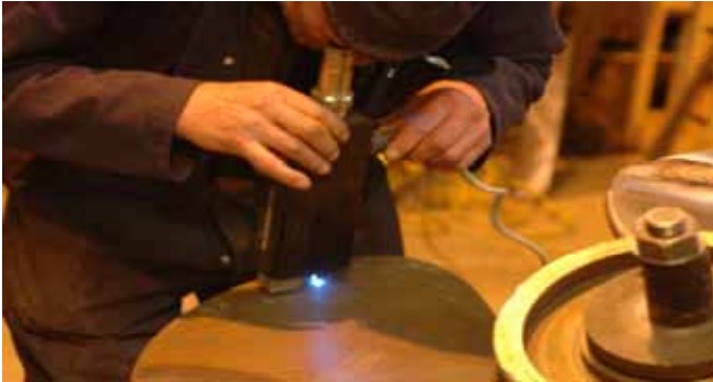
Using a portable Spectroscope to determine the propeller material specification
