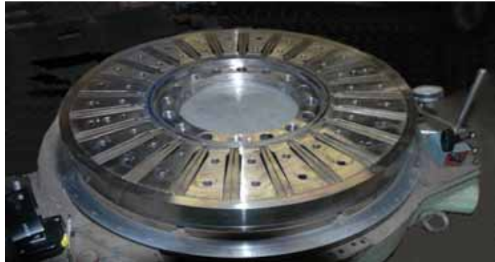
Geislinger Damper during concentricity checking On final assembly following servicing/overhaul
